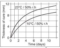
Diagram 1: Curing speed Sikaflex®-252
