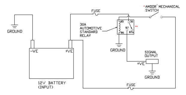
\*AMDOR MECHANICAL SWITCH RATED FOR A MAXIMUM CONTINUOUS DRAW OF 1.5A @12VDC \*\*RELAY IS NOT INCLUDED WITH AMDOR MECHANICAL SWITCH
